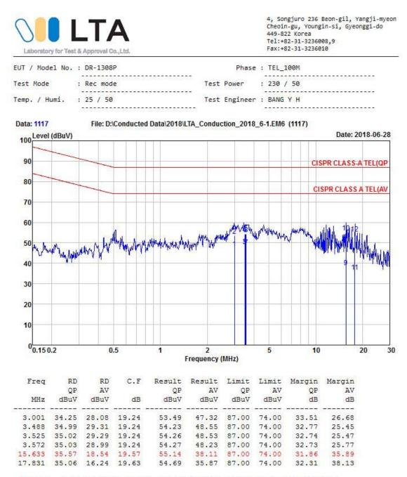
Remarks: C.F (Correction Factor) = Insertion loss + Cable loss + Pulse Limiter
